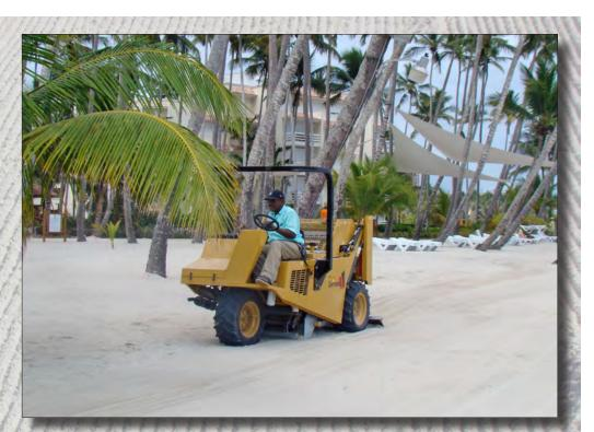
The Cherrington Model 3000 is ideal for resort beaches. The three-wheel design, zero-turn capability, low profile, and short overall length allow you to quickly screen-clean along boardwalks; around cabanas and furniture; and under low hanging trees.
