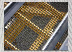
Choose from interchangeable screens from 3/8" (10mm) to 1" (25mm) to quickly remove everything larger than the selected screen hole size.
